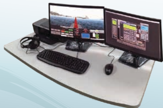
Desktop configuration with ShipSim + GMDSS simulator
